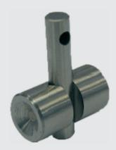
The tribosystem consists of the two V-blocks, made of the tested material, pressed at the constant or increasing load P against the journal that rotates at the constant speed n. Experiments may be carried out under conditions of dry friction. The friction contact may also be lubricated by a grease or solid film lubricant - deposited once before a run, or lubricated by an oil poured into the reservoir, after the immersion of the test specimens in the oil.
