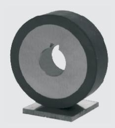
The test involves the abrading of the test specimen (plate), made of the tested material, with an abrasive that is introduced between the plate and the rotating wheel having a rubber rim. The plate is pressed at a specified force against the wheel rotating at a defined speed n. Before and after the run, the plate is weighed and then its mass loss is calculated. The result is related to the one obtained for the reference material.
