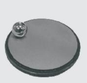
The tribosystem consists of the stationary pin (ball) pressed at the required load P against the disk rotating at the defined speed n.
