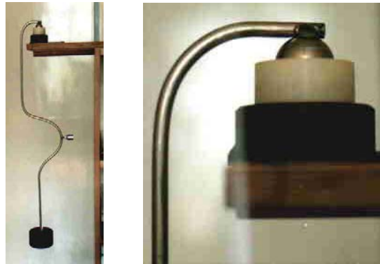
Fig. 5. Test rig for the evaluation of oscillating coefficient of rolling friction
